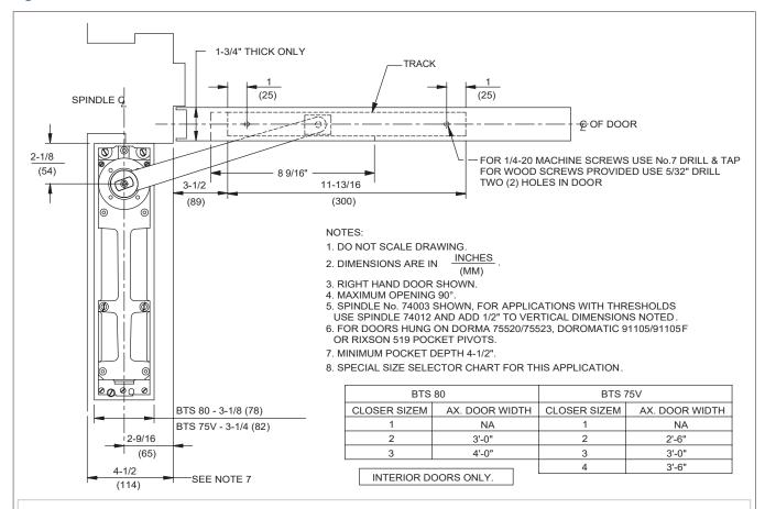
FLOOR CLOSER MODEL: BTS 75V/P, 80/P WITH 7451N SLIDE ARM ASSEMBLY POCKET PIVOT APPLICATION (PULL SIDE MOUNT)
